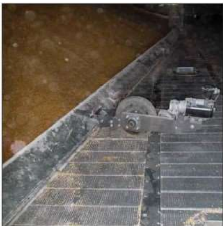
The V1 automatic push tractor measures 11 inches wide and models range in weight from 100 to 145 lbs.
