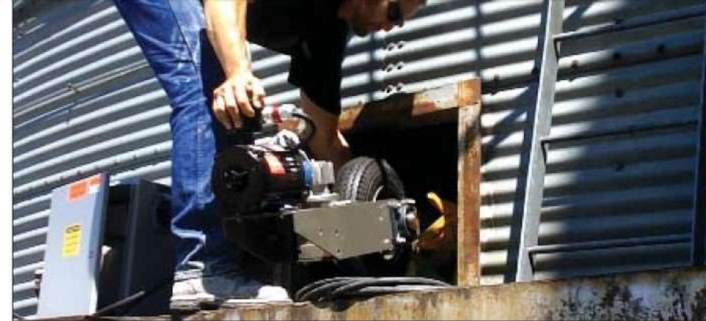
The V1 automatic push tractor is able to fit into any bin door.
